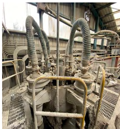
Figura 3. Hidrociclones de 10 Pulgadas (254 mm). Figure 3. Hydrocyclone of 10 inches (254 mm).
