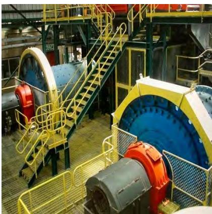
Figura 2. Molino de Molienda Primaria 9x13 pies (2.74 x 3.96 m). Figure 2. Primary milling mill 9 x 13 ft. (2.74 x 3.96 m)
