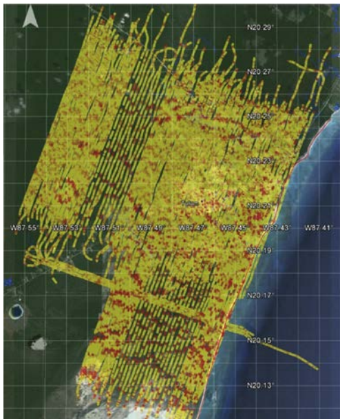
Figure 6: 7200 Hz channel of 2007 and 2008 surveys after drift correction, height reduction and destripping (Google Earth © map with overlay).
