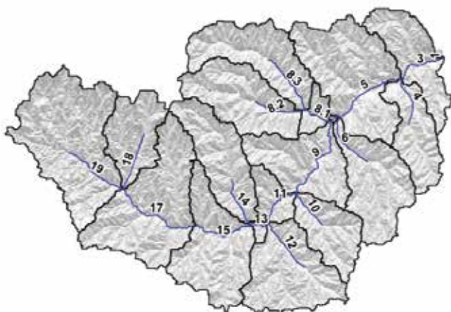
Figure 5. The Pfafstetter numbering scheme for the Little Washita watershed, Oklahoma (U.S.). The figure shows an example of the Pfafstetter river-network numbering.
